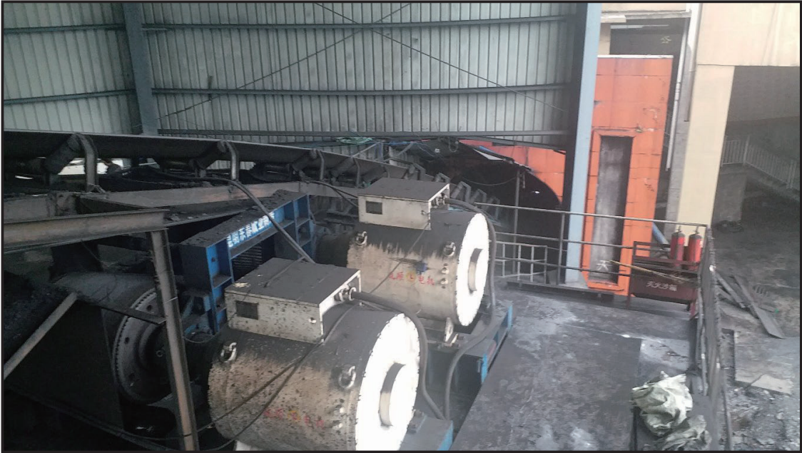
Figure 9-2: Main Decline installed with the main conveyor of the Xiejiahegou Coal Mine
