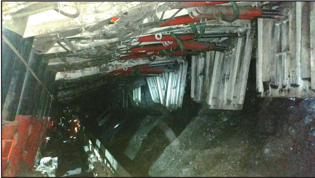
Figure 9-7: Longwall retreat mining at the Xiejiehegou Coal Mine
